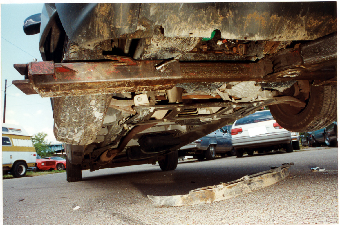
36. Close up view of damage to the lower surface of the bumper fascia.
